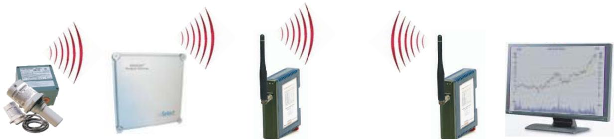
Reliable wireless communications is a key requirement, since this system is a retrofit in any existing facility. The cost of running wire is prohibitive in many locations. The ioPro WDL robust 1 Watt, 900 MHz Frequency Hopping Spread Spectrum (FHSS) radio communications link is immune to electrically noisy facilities and provides reliable communications between the remote units and the master. It can also be deployed as a repeater in environments where required.
