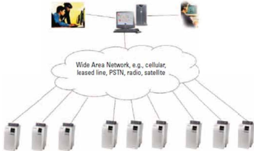
An RTU design must assume a less reliable, low speed network with a higher connection cost and higher, operating cost, all of which encourage the user to minimize the amount of data that is transferred over the network. This incurs more ramifications than engineers may, at first, consider.
