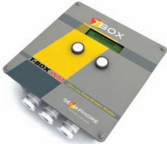
*The fully integrated, IP66 weatherproof housing is available in aluminum or stainless steel. This ready-to-install solution includes single or redundant lithium batteries, PSTN or wireless communication device, I/O for end device interfacing, and optional liquid crystal display.*
