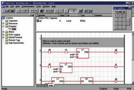
*T-BOX processing capabilities are appropriate to automation requirements as well as custom calculations and logic. The LD programmer will find the IEC 61131-3 ladder diagram editor to be familiar and intuitive. For those who prefer structured text, a BASIC environment is also provided. Systems suppliers who use Microsoft tools are also supported through Microsoft Automation.*
